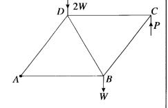
Draw a stress diagram using Bow's notation and hence, find the stresses in the rods stating whether they are tensions or thrusts.
